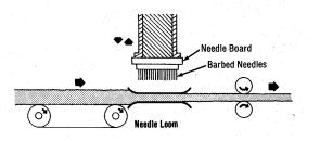
arrangement. By varying the strokes per minute, the advance rate of the batt, the degree of penetration of the needles, and the weight of the batt, a wide range of fabric densities can be made. For additional strength, the fiber web can be needled to a woven, knit, or bonded fabric. Bonding agents may also be used.
