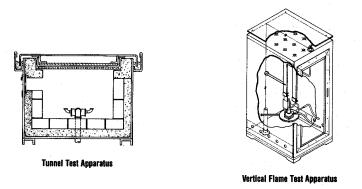
**Vertical Flame Test:** A test for flame resistance in which a specimen is mounted in a vertical holder and exposed to an open flame for a specific time. The open flame is then extinguished and continued flaming time and char length of the sample are measured.
