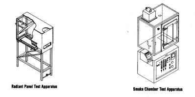
**Smoke Chamber Test:** This method assesses the smoke generating characteristics of a sample due to pyrolysis and combustion by measuring the attenuation of a light beam by smoke accumulating in a closed chamber under controlled conditions. Results are expressed in terms of specific optical density.
