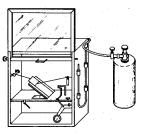
Diagonal Flame Test Apparatus
