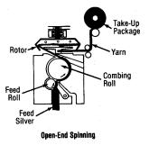
process, in a sense combines the traditional processes of roving and spinning in one operation. Present work is directed toward incorporating the drafting operation into the process by using card sliver as the feedstock. This can facilitate process linking.
