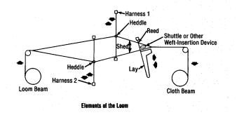
**LOOM BARRÉ:** A repeated unevenness in the fabric, usually running from selvage to selvage, and caused by uneven let-off or take-up or by a loose crank arm.
