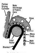
Sanforizing Method of Producing Shrinkage
